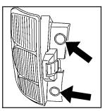
Remove the taillamp screw covers and then remove the two screws.
